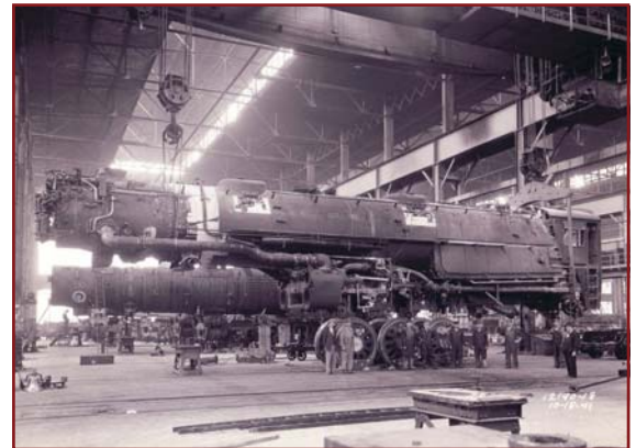
A Rio Grande Railroad 4-6-6-4 locomotive having its wheels applied in the Baldwin Erecting Shop in 1941
